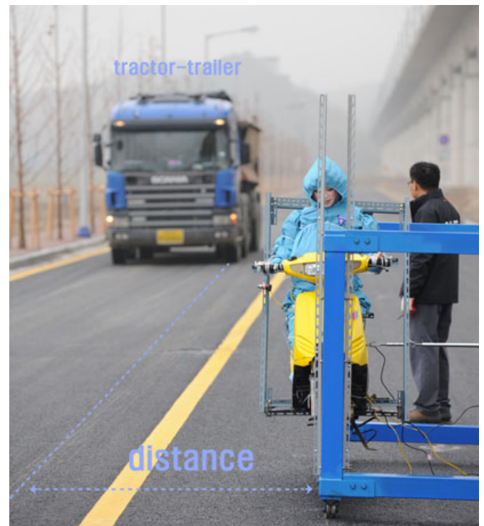
FIG. 4—Photograph of the test site. The experiment was performed along a straight road where the tractor-trailer could accelerate and steadily maintain the test speed.
